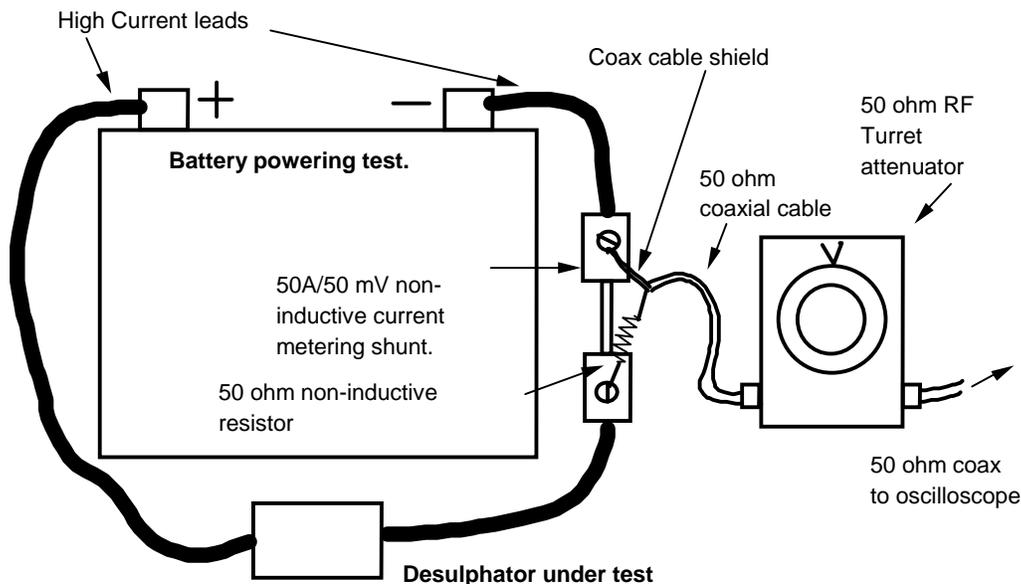
**Appendix 1 Fig 2 Current pulse measuring set up for the de-sulphator.** The high current lead connecting the negative post of the battery to the metering shunt should be as short as possible, as this is the “common” or ground of the system. Lengths of coaxial cables between the measuring shunt and the attenuator should be no more than 1 meter.
