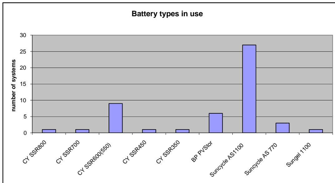
**Fig 21 Battery types encountered during the survey.** As is evident, the battery types installed are primarily flooded lead acid cells, with one example of a gel-cell system (Sungel 1100). The Century Yuasa SSR series batteries are lead-calcium tubular plate construction, the remainder are lead antimony construction. Most systems have battery capacities in excess of 600AH (C100 rate). 24V.
