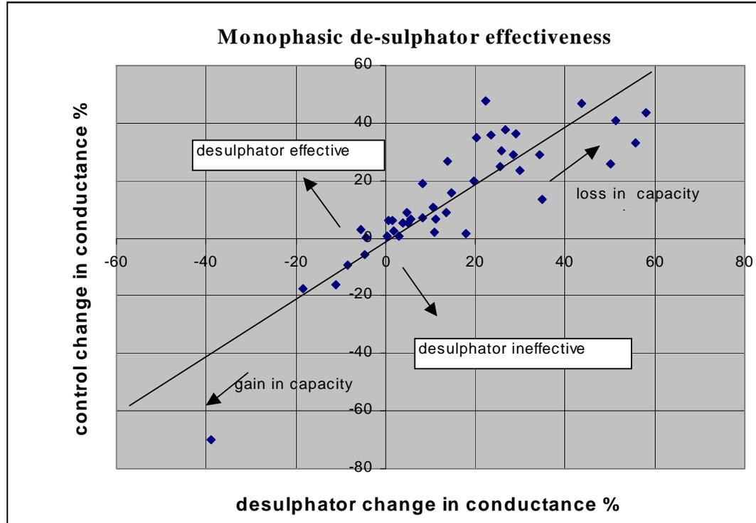
**Fig 11 Plot of conductance changes in the test battery population** resulting from the application of the monophasic pulse de-sulphator.
