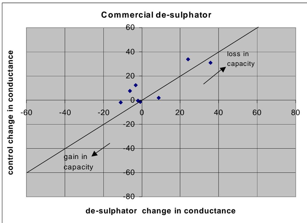
**Fig 12 Plot of conductance changes in the test battery population** resulting from the application of the commercial sweeping pulse de-sulphator. Unfortunately only 8 could be installed, so the performance of this population and the preceding population could not be statistically compared. However, the pattern is much the same suggesting that it was also somewhat effective.
