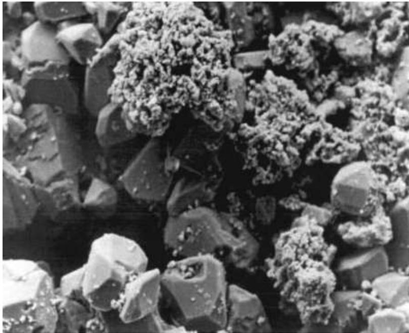
**Fig 2** This is a electron microscope picture, magnified 549 times, of a 6 month old battery positive plate used in an ambulance. Given the amount of sulphation, this battery has already reached the end of its service life. Note the large sulphate crystals on the battery plate and the severe erosion of the sponge lead plate material. This battery was never de-sulphated.
